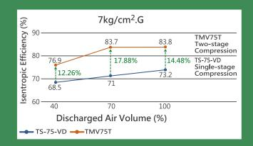
The traditional two-stage gear-shift design only has the best compressing efficiency at its fixed setting-pressure. It's difficult to maintain the best efficiency when the air consumption or pressure is changed.
